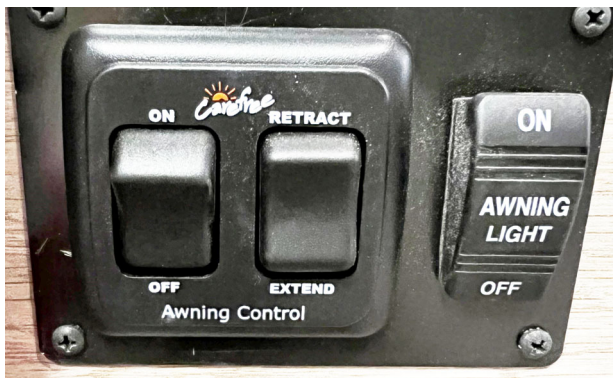
Power Awning control switches and Awning Light Switch (Located near the entrance door) -Typical View
