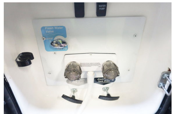
Exterior Shower/Wash Station –Typical View
