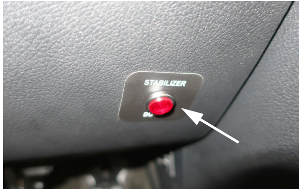
“Stabilizer Down” Light (Located on lower dash) -Typical View
